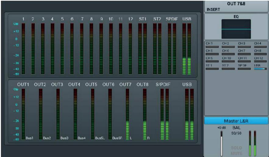
The left side of the page gives a complete overview of all the inputs and outputs of the console, the right side shows the Master L/R output band, whose functionality exactly follows the 7-8 stereo buses.
