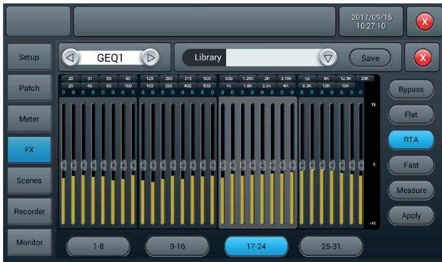
When the measurement is complete, the Measure button turns off. Now close the GEQ page and insert the GEQ into the L&R bus either via the effects page or in the input section of the L&R bus. Then go back to the GEQ, lower the Master fader and click Apply, which will change your faders to equalize according to the last bar.
