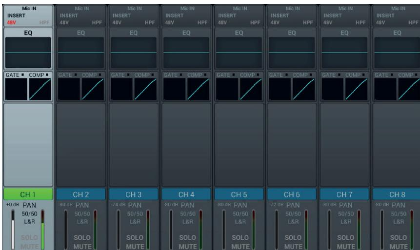
Enter the effects section in the Setup dialog box and choose GEQ1 or GEQ2 and enable RTA. Note that there are two normal modes (below) and others that will show small changes more clearly. The mode you use doesn't matter here.
