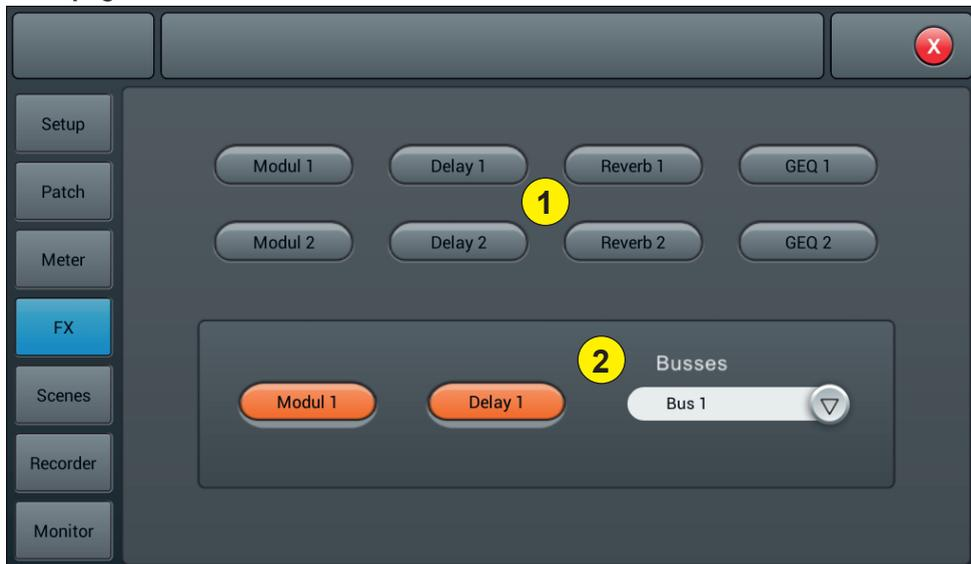
The effects consist of 8 modules, which are: 2 Modulations, 2 Delay, 2 Reverb and 2 15-band graphic equalizers. Each module can only be inserted once into an input processing channel or bus processing channel. You can insert up to two effects into a bus or channel. For example reverb & delay to create a vocal effect.
