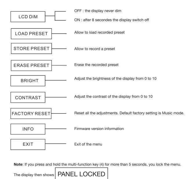
To unlock the menu, press and hold the multi-function button again for more than 5 seconds.
