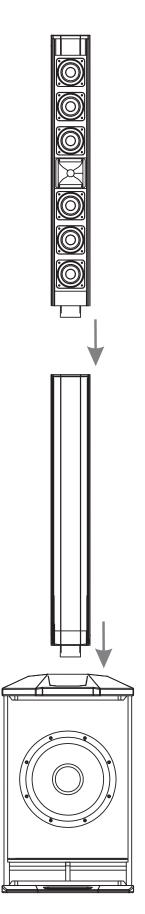
The MOJO1200Line column is directly mounted above the subwoofer thanks to its contact slot.
