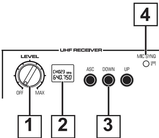
**A1** - Volume control knob for the HF module. From OFF to full power (clockwise).
