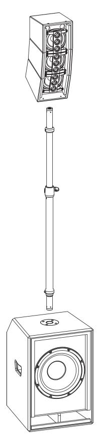
The MOJO2200curve satellite is directly mounted above the subwoofer thanks to its contact slot.
